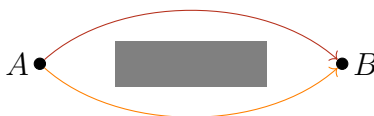
Figure 2.2: Multiple paths from point A to B exist, but the optimal policy under \ell^2 -loss converges to the prohibited middle path. This is because the distribution is unimodal.
