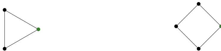
Figure 15.1: The two green nodes have the same computational graphs and therefore the same embedding despite having different neighbourhood structures.
