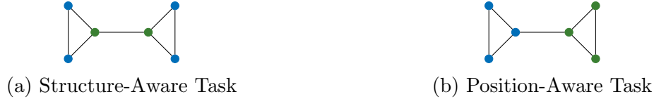
Figure 15.2: Structure and Position Aware Tasks; GNNs often work well for structure-aware tasks but fail at position-aware tasks.
